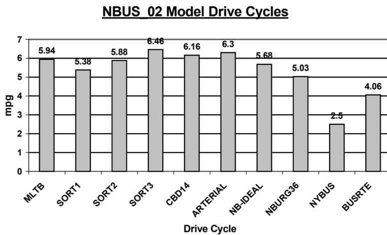
Fig 10: NBUS\_02 model drive cycle results
