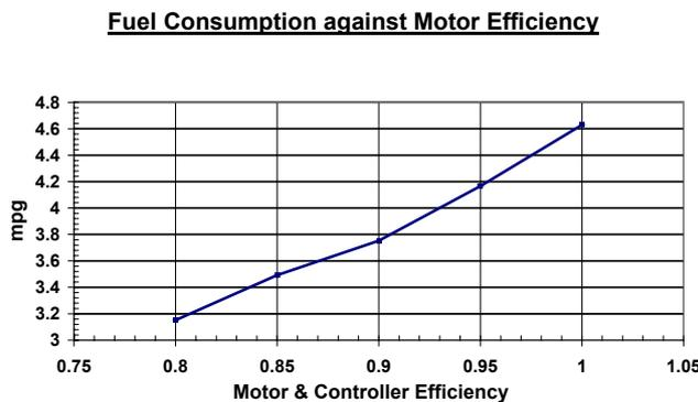
Fig 3: Mpg against Motor Efficiency
