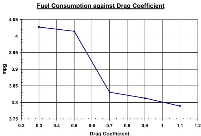
Fig 9: Mpg against Drag Coefficient
