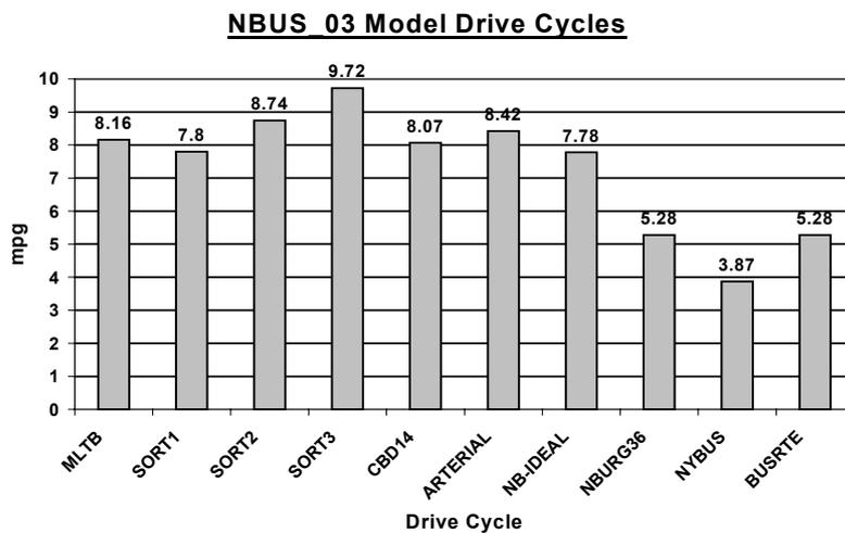
Fig 11: NBUS\_03 model drive cycle results
