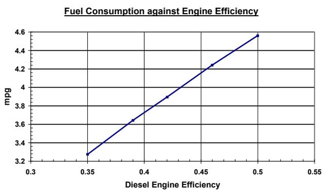
Fig 1: Mpg against Diesel Engine Efficiency
