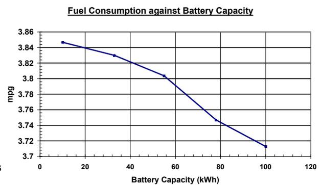
Fig 4: Mpg against Battery Capacity
